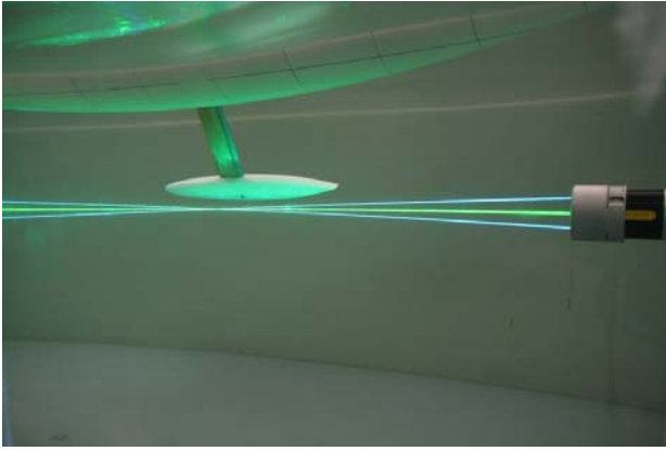
Figure 8: LDA measurements in wing sectional plane
